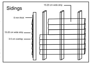
C Studs or timber studs, 2 feet or 610mm apart can be screwed to the structure. The installation can be done with an over lap of 30 to 50 mm.
