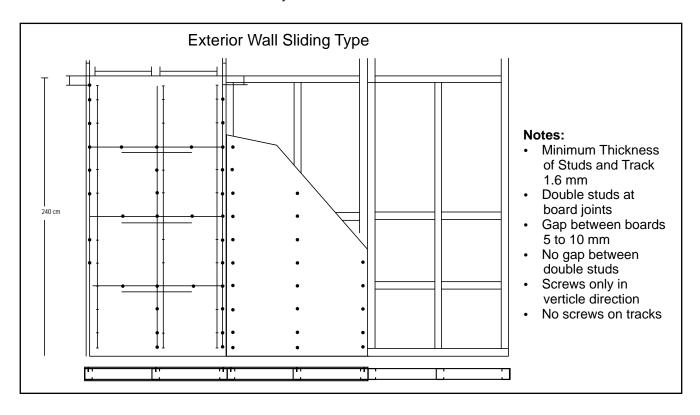
The galvanized studs and tracks should have a thickness of 1.6mm or 2 mm.
