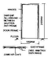
Half an hour fire resistant doors with Bison Board have been successfully tested at the Central Building Research Institute Roorkee. Shutter Frame is made out of hard wood with top, bottom, middle & intermediate rails and two vertical members, providing an air gap of about 25 mm. Bison Panels 12 mm thick, protected with a special coating are fixing on either side of the shutter frame.
